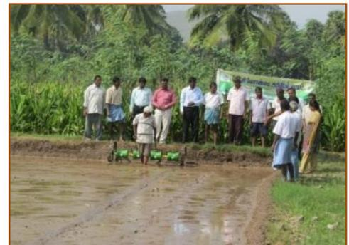
The KSNM direct paddy seeder covers 8 rows of 20 cm row to row spacing at a time. This implement ensures uniform plant population throughout the field. This hyperboloid shaped drum with 200 mm diameter, 9 numbers of seed metering holes of 9 mm hole diameter. Baffles are provided inside the drum between seed holes resulting in uniformity of seed rate throughout the operation. These baffles also
